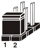
Jumper Block 1-2 pin close(enabled) Looks like this
