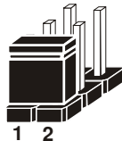
Jumper Block 1-2 pin close(enabled) Looks like this
