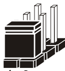
Jumper Block 1-2 pin close(enabled) Looks like this
