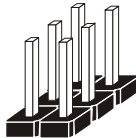
Jumper Block looks like this
