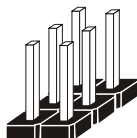
Jumper Block looks like this
