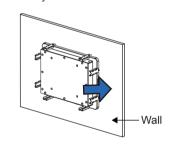
Step 3. Install 8 hooks onto the mounting brackets on the four sides of the LCD monitor to secure firmly.
