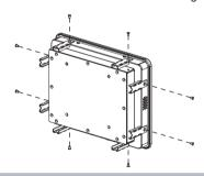
Step 2. Mount the LCD monitor equipped with 8 brackets onto the wall firmly.
